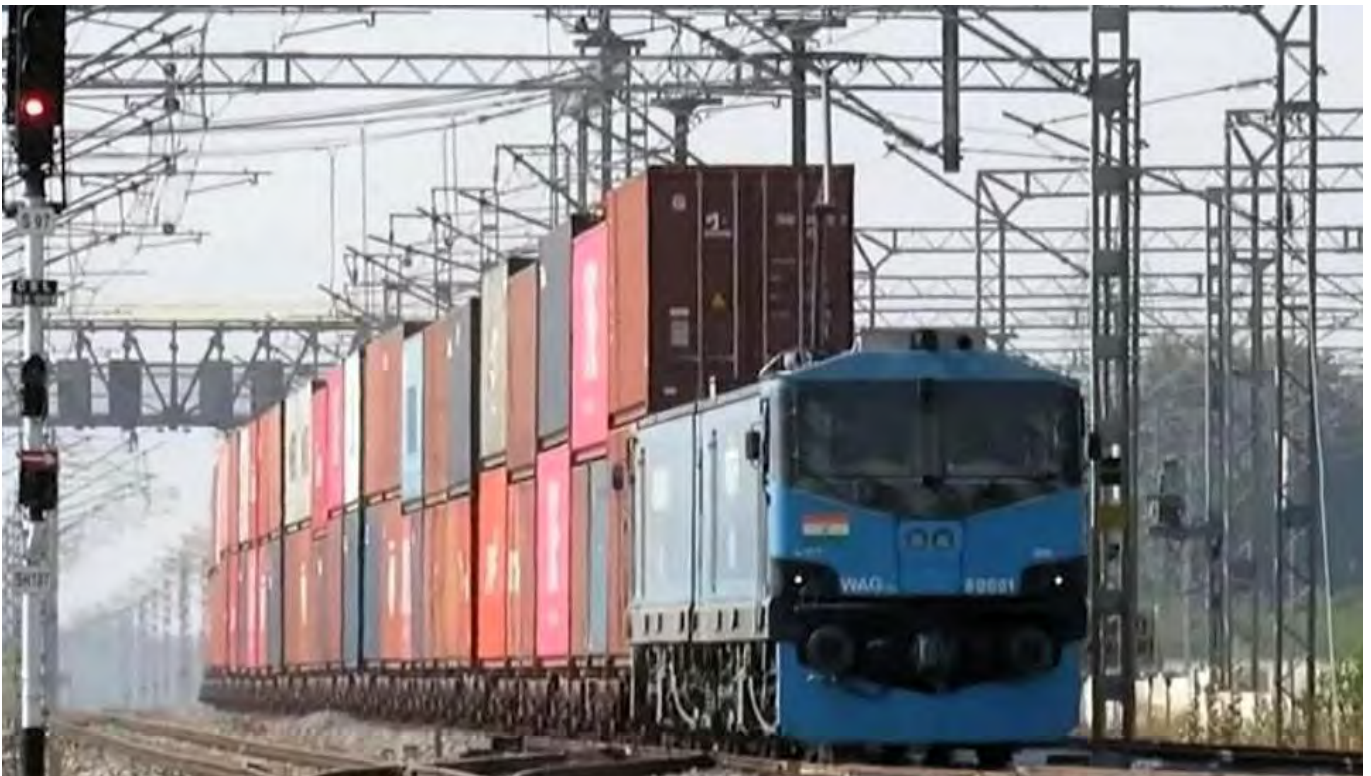
Figure 4-2: Double stacked container trains are typically the type of freight trains that will share the standard-gauge corridors with regional rapid transit
