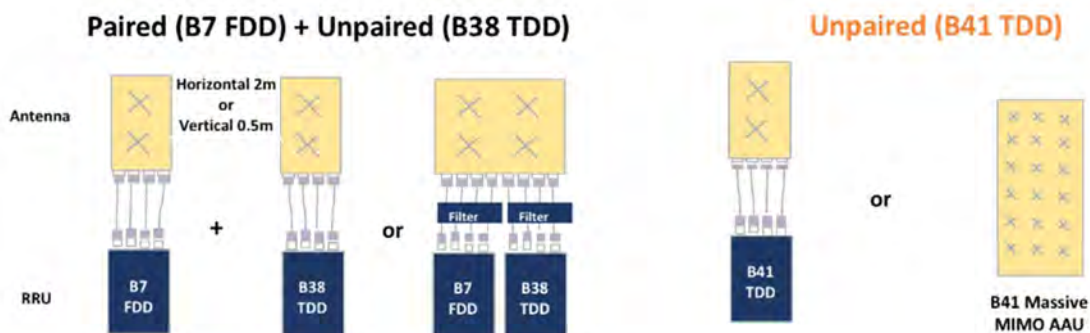
Figure 34: Comparison of FDD and TDD Deployment
