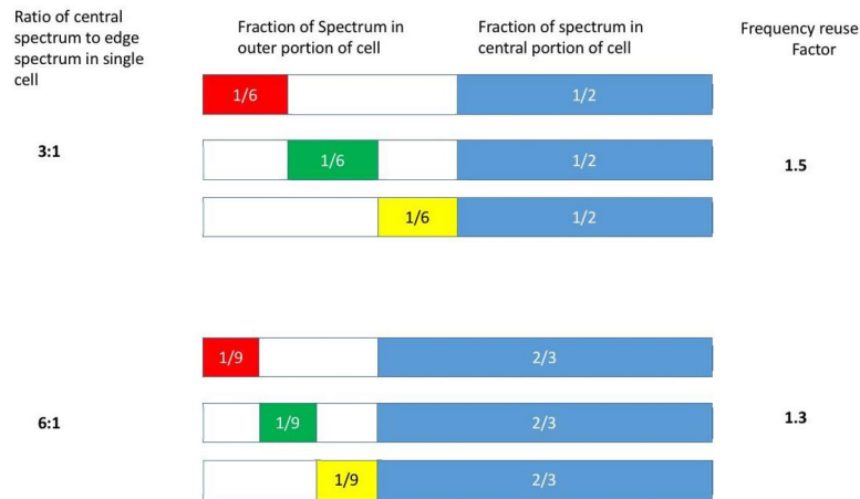
Figure 8: Different ratios of central to edge spectrum for strict FFR
